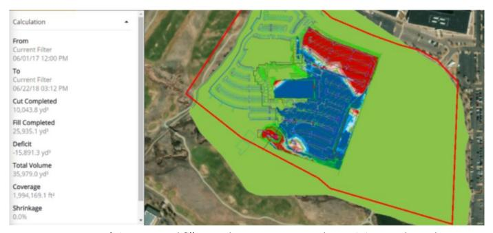
Real time cut and fill map shows progress and remaining earth-works
