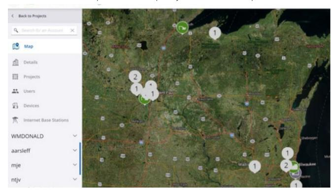
Telematic's can be used to show real time location of every connected machine.
