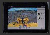
Factory fitted 10" rear view camera and slope control interface.
