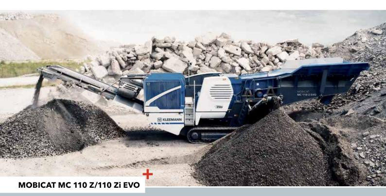
The MOBICAT MC 110 Z EVO has an independent double-deck prescreen, which effectively screens the fines in the feed material. The machine is impressive in individual applications or interlinked with an MCO 9 EVO cone crusher or a MOBISCREEN MS EVO screening plant.
