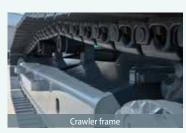
Special crawler frame design is easily cleaned of mud.
