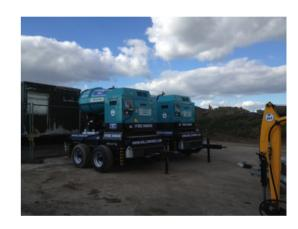
Our most popular unit is the De Dust 75 all in one. With a built in 2000 litre water bowser and an on-board generator it turns up ready to work with no need for trailing cables and hoses. Fitted on a site towable chassis it is easy to manoeuvre around site as the project progresses. Fitted with remote oscillation it is simple to set up the area of coverage as required. With a throw of up to 40 meters it provides plenty of coverage for most sites.
