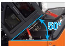
The engine cover slides up and down for easy servicing in confined space. The cab floor can be tilted up to 50° for easy access to the floor bottom and engine rear.
