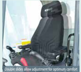
Double slides allow adjustment for optimum comfort
