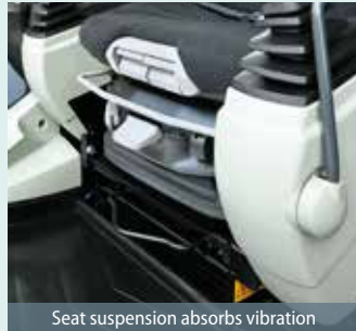
Seat suspension absorbs vibration
