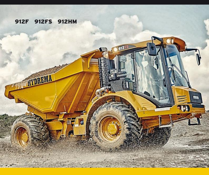
A unique combination of articulated center pivot, wide wheels and high ground clearance - for superior off-road performance.
