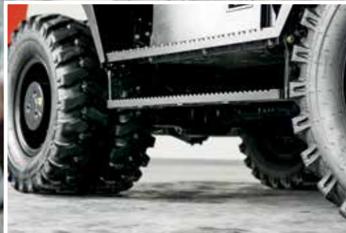
High ground clearance reduces damage from obstacles.
